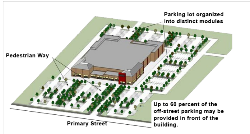
Figure 5.7.F(5): Large Retail Parking Lot with Over 200 Spaces
