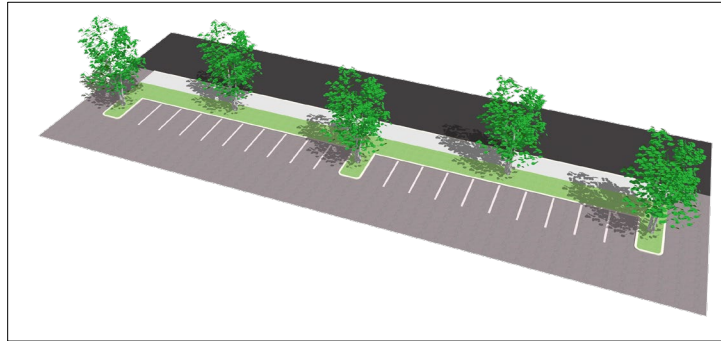
Figure 5.3.H(5)a.1(b): Interior Parking Area Minimum Plantings
